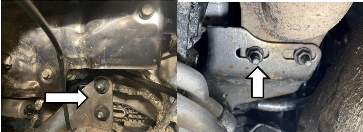
**Note:** Make sure the battery is not connected since the shield can short the starter motor located above the sensor.
