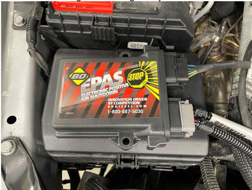
6. Carefully secure all wiring within the engine bay with supplied wire ties to that it is away from moving parts, chafe hazards and heat sources. Use extra care with the crankshaft position sensor wiring due to the close proximity to belts, fans and road debris and potential consequences of a short or break in this wire.
